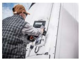
uses a thermal camera module to observe analog equipment. A custom machine learning model is created to train the device to recognize normal thermal data from the system and pump that data to a cloud service using the Blues Wireless cellular Notecard System on a Module.
